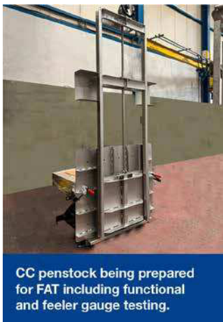
Highest quality welding, subject to 100% visual and dye-penetrant NDT, with client witness hold points at every stage.
